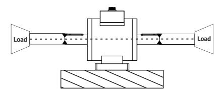
DON'T WELD MATING COUPLER TO TORQUE SHAFT
