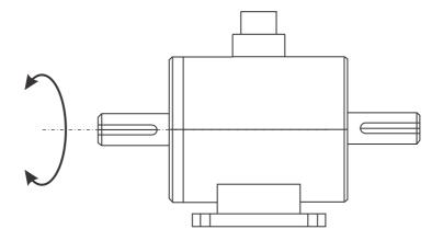
Torque must be in center in-line of axis whether its clockwise (or) anti-clockwise direction
