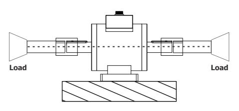
ENSURE THE MOTOR SHAFT, TORQUE SHAFT & LOAD SHAFT TO BE IN PERFECT ALIGNMENT
