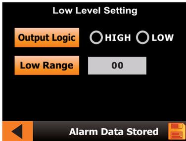
Output logic - select **HIGH** for energizing the relay below the values. Till then the relay will be de - energized.
