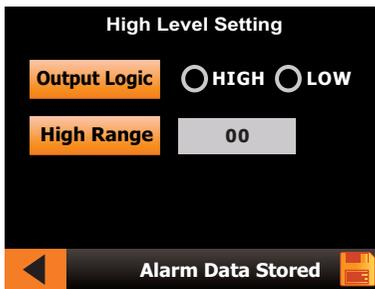
**Output logic** - select **HIGH** for energizing the relay after the values. Till then the relay will be de - energized.
