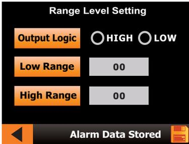
Output logic - select **HIGH** for energizing the relay between the set values. Till then the relay will be de -energized.
