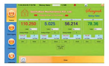
Real time value of 3 load cell and a displacement sensor with peak and zero option
