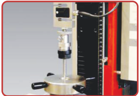
S-type load cell in puncture resistance force testing
