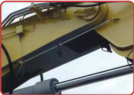
Magnetic cursor potentiometer for construction equipment to precisely measure the arm movements
