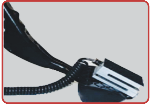
In-vehicle pedal effort sensor for automotive brake & clutch testing
