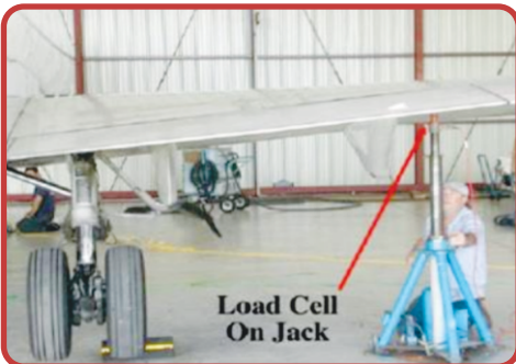
Hydraulic jack lift force feedback monitoring using load cell in avionic applications
