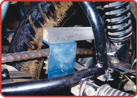
Two wheeler chain tension monitoring system
