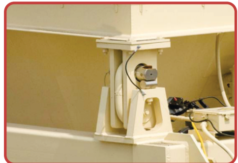
Pin type load cell in asphalt dispensing hopper weighing
