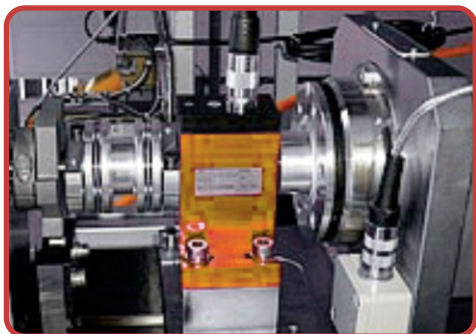
Rotary torque transducer in automotive pump testing
