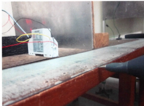
Electrostatic Discharge Immunity Test Setup (Contact Discharge)
