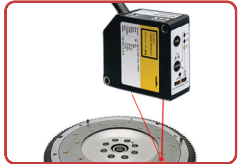
Non contact Laser displacement sensor used to measure flatness of auto components
