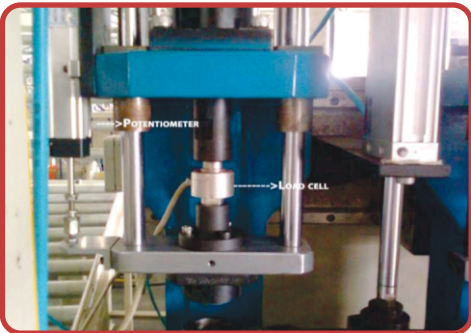
Axial load cell in bush pressing press assembly
