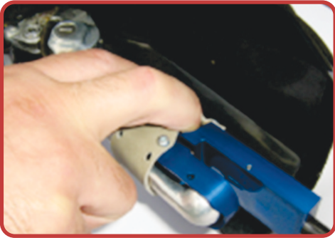
2 wheeler & 3 wheeler clutch / Hand brake effort sensor for in vehicle clutch force measurement
