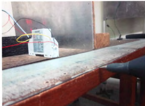
Electrostatic Discharge Immunity Test Setup (Contact Discharge)
