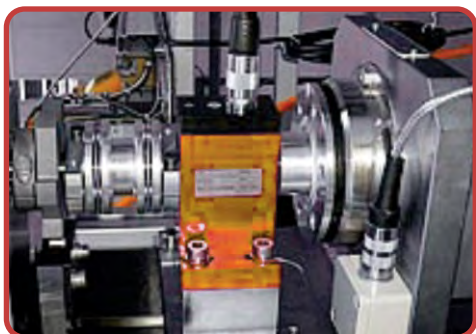
Rotary torque transducer in automotive pump testing
