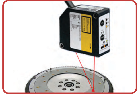
Non contact Laser displacement sensor used to measure flatness of auto components
