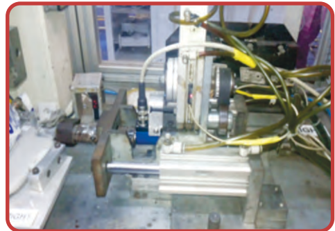
Rotary torque transducer kept inline in sun visor assembly to ensure assembly torque quality
