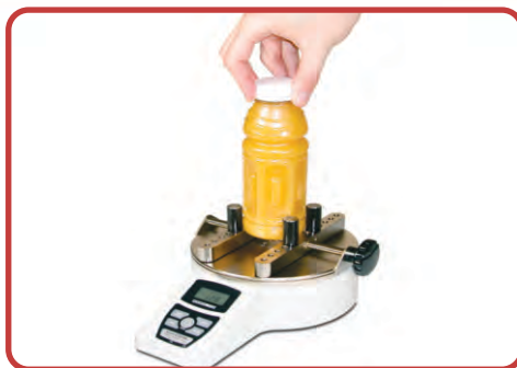
Bottle cap torque testing using customized reactive torque transducer
