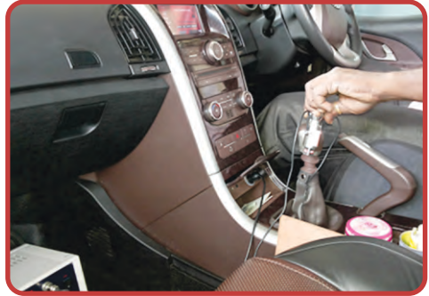
In-vehicle automotive 2 axis gear effort force sensor with indication & logging systems
