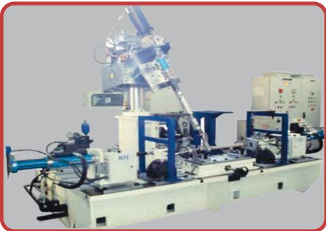
Rotary torque transducer kept inline with steering column simulator in steering rack and pinion assembly test rig
