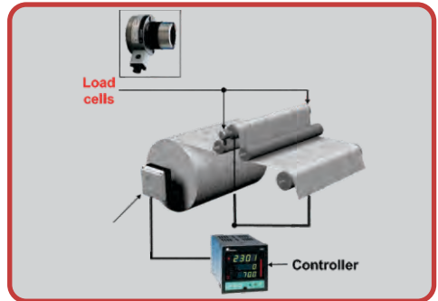
Radial type load cell for web tension monitoring in textile and paper industries monitoring
