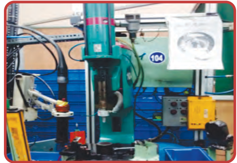
Actuator load measurement in the oil seal tear machine
