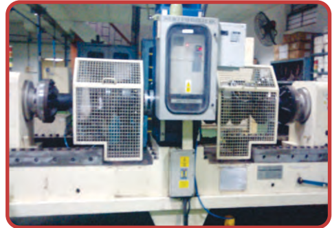
To measure the torque acting on the brake chamber in the double end fatigue rig
