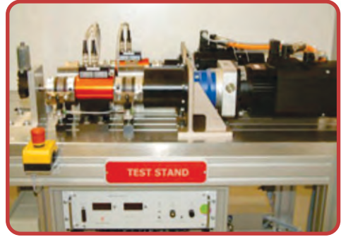
Rotary torque transducer with RPM output in seat regulation DC motors test rig
