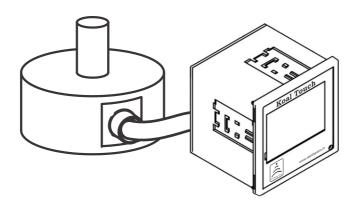
In an environment with a high amount of moisture or humidity, create a drip loop on the cable to prevent any water from flowing into the sensor.
