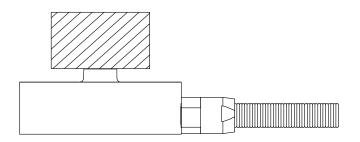
• Fixture must not contact diaphragm area.
