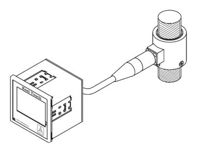
In an environment with a high amount of moisture or humidity, create a drip loop on the cable to prevent any water from flowing into the sensor.
