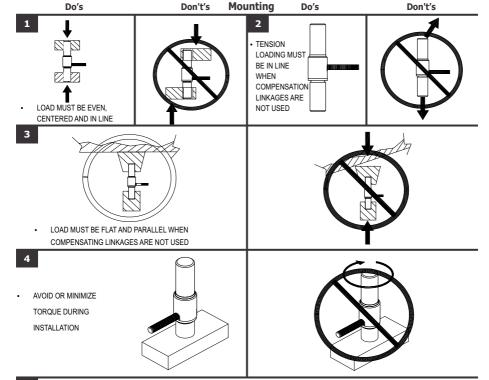
ROD END BEARINGS WITH CLEVISES OR ALIGNMENT COUPLERS MAY BE USED TO MAKE UP FOR MISALIGNMENT
