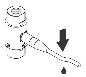
• Make connection according to color code of sensor connection to amplifier.
