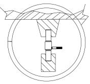
LOAD MUST BE FLAT AND PARALLEL WHEN COMPENSATING LINKAGES ARE NOT USED
