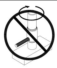
ROD END BEARINGS WITH CLEVISES OR ALIGNMENT COUPLERS MAY BE USED TO MAKE UP FOR MISALIGNMENT
