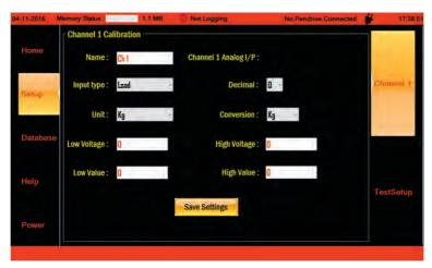
Calibration setting of load cell and its units conversion
