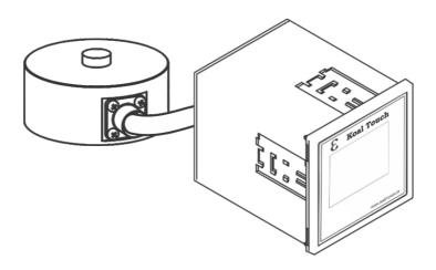
In an environment with a high amount of moisture or humidity, create a drip loop on the cable to prevent any water from flowing into the sensor.
