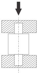
Load must be flat and parallel when compensating linkages are not used
