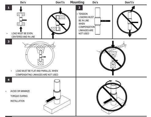
PROD END BEARINGS WITH CLEVISES OR ALIGNMENT COUPLERS MAY BE USED TO MAKE UP FOR MISALIGNMENT
