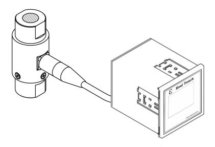
In an environment with a high amount of moisture or humidity, create a drip loop on the cable to prevent any water from flowing into the sensor.
